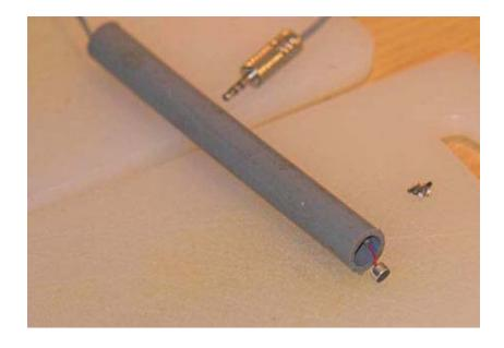
The capsule fitted to the wire is now threaded through the tube,
